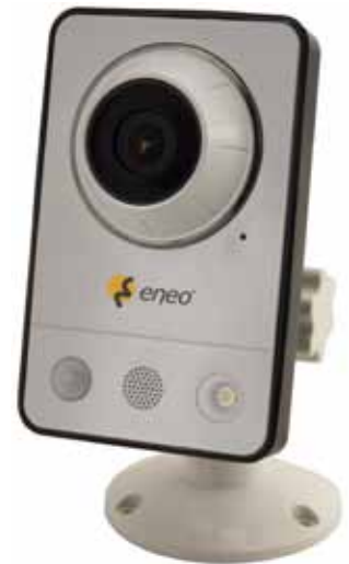
Art.: 204288 1/4" Network Camera, H.264, 2DNR, 1600x1200, 3,6mm, 5VDC, PoE, ONVIF
